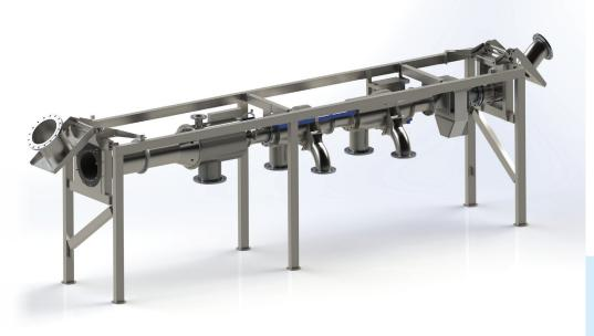
The FLS Delousing System is a market-leading solution for removing salmon lice. We deliver high-quality Norwegian technology and optimum fish welfare - at a competitive price. In our modular design, each line is operated separately, and it is easy to increase the capacity of the installation by simply adding lines.
